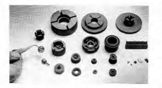
PIECE PARTS of alumina oxide ceramic (AL<sub>2</sub>O<sub>3</sub>), machined in "bisque" state, retain their precise shapes although shrinkage during firing may have been as much as 17 percent.
